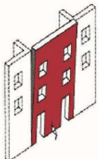
Mechanism type A: overturning of the façade
