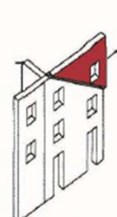
Mechanism type H: in-plane failure, diagonal crack
