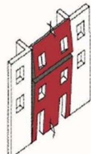
Mechanism type F: vertical arch effect associated with ties at the top of the façade
