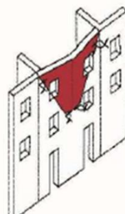
Mechanism type G: horizontal arch effect
