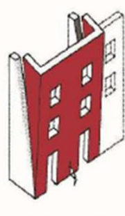
Mechanism type B2: overturning of the façade and two party walls
