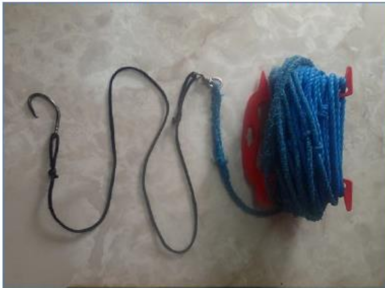
Broken fluorocarbon leader; Broken Owner Mutu hook
