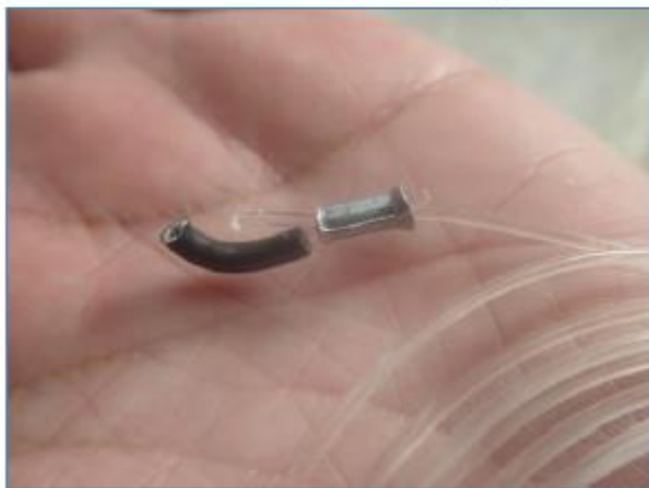
Broken fluorocarbon leader; Broken Owner Mutu hook
