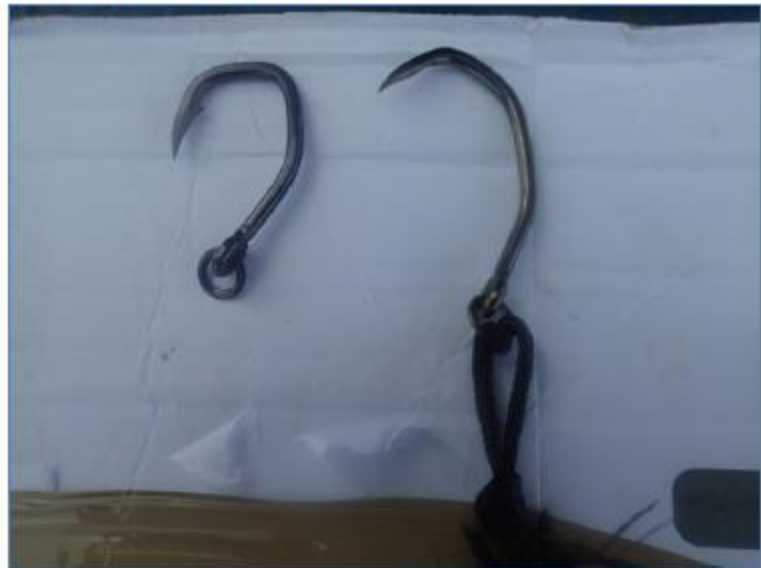
Modified hand-line fishing gear with 3,5 mm rope; Banded VMC hook
