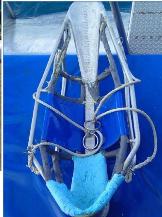
Aluminum cradle; rigid stainless steel tagging platform fixed inside of the cage frame.
