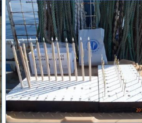
Aluminum cradle; rigid stainless steel tagging platform fixed inside of the cage frame.
