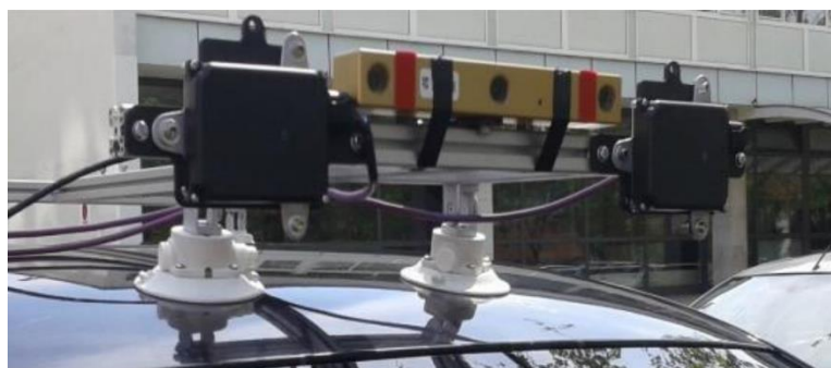
Stereo vision and radars fusion (car driving in Zagreb)
