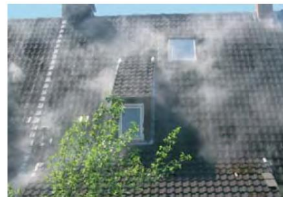
Smoke pressed out by a Blower Door fan to show the roof leaks
